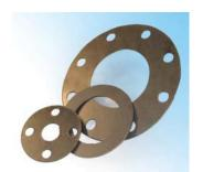
Pure exfoliated graphite with a stainless steel foil reinforcement for improved handling and load-bearing characteristics. The excellent conformability of graphite means that the material is suitable for applications where bolt load is limited or flanges are damaged.
